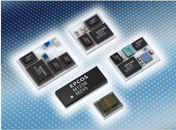
Fig. 1. Front-end module for mobile phones before encapsulation to a system in package.
