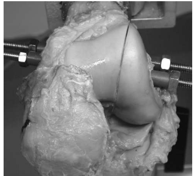
Figure 1. Relocated osteotomy of the lateral femoral condyle. The defect of the saw blade is compensated for with a Teflon film.
