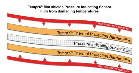
TemprX® is a thermal protection polyimide film for use with Pressure Indicating Sensor Film in applications that reach high temperatures. Pressure Indicating Sensor Film is thin, flexible, and instantly captures and records pressure distribution and magnitude between any two contacting, mating or impacting surfaces. It is simple to use, effective and inexpensive.
