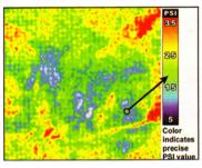
Pressurex Zero pressure-indicating sensor film characterizes tactile contact surface pressure down to 7.2 psi. The easy-to-use flexible film is placed between
