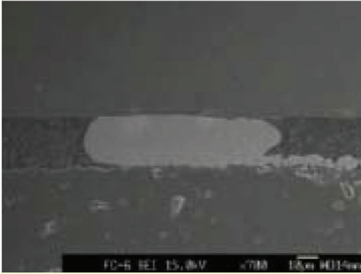
Figure 5. Cross-section of a gold stud bump, with the top surface flattened by pressure.
