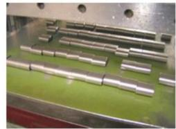
Bryan inserted the film which he had ordered in Super Low pressure range of 70--350 PSI (5--25kg/cm²) between the press plates during a product run and saw the uneven distribution of pressure between the capacitors. As a result, he could prove the press plates weren't flat and were causing uneven pressure distribution.
