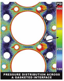
Sensor Products' Pressurex calculates surface pressure by creating an instantaneous color profile. The varying color intensities correlate to pressure ratings such as in this gasket assembly, where it can be used to illustrate how surfaces engage and deform under stress — displaying sealing flaws and inconsistencies.
