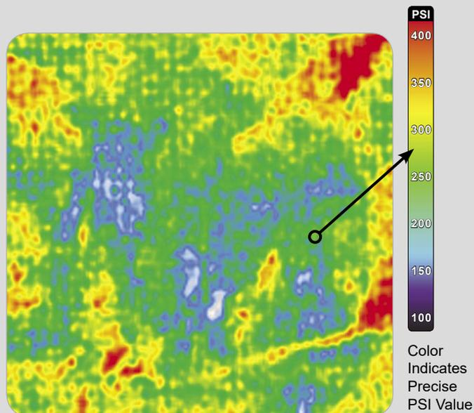
The image to the left depicts a Fujifilm Prescale® impression, while the image to the right is a color mapped version produced with the Topaq® Tactile Force Analysis System.
