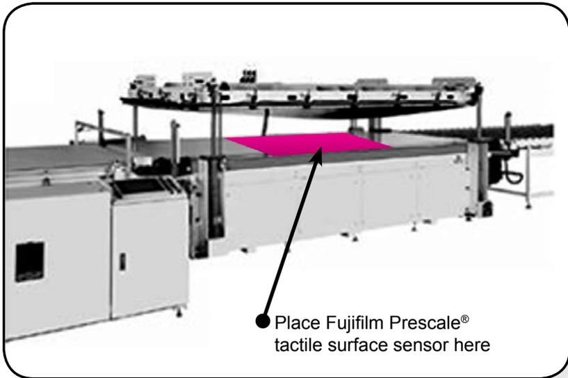
**2** Instantaneously and permanently the film captures both the pressure distribution and magnitude that occurs between the contacting surfaces.
