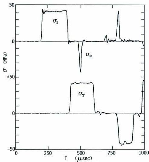
Fig.4 Incident, reflected, and transmitted Stress waves in tests
