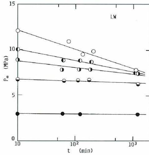
Fig.7 Change in pressure sensitivity after elapsed time
