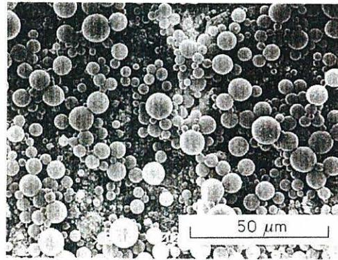
Fig.2 Microstructure of "Prescale" by SEM
