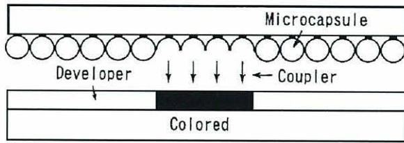
Fig.1 structure and mechanism of pressure Sensitive film "Prescale"
