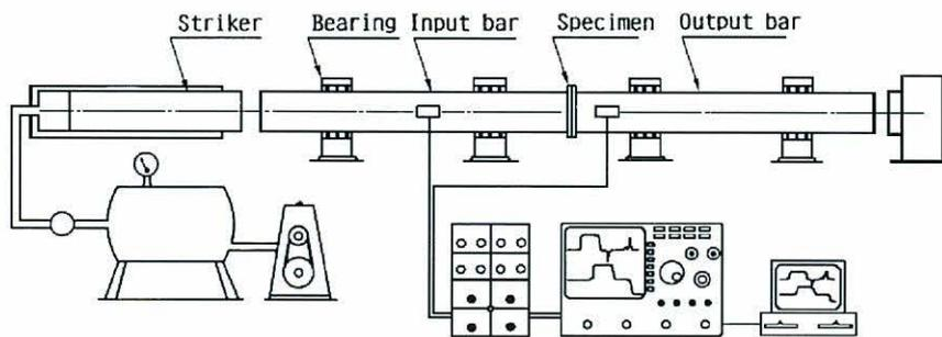
Fig.3 Compressive split Hopkinson bar apparatus and measuring circuit
