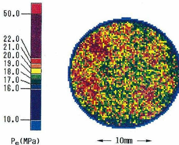
Fig.5 Colored impression digitized by electronic densitometer
