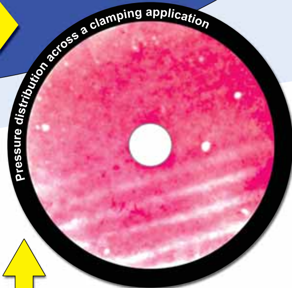
Fujifilm Prescale® film BEFORE Topaq® Analysis
