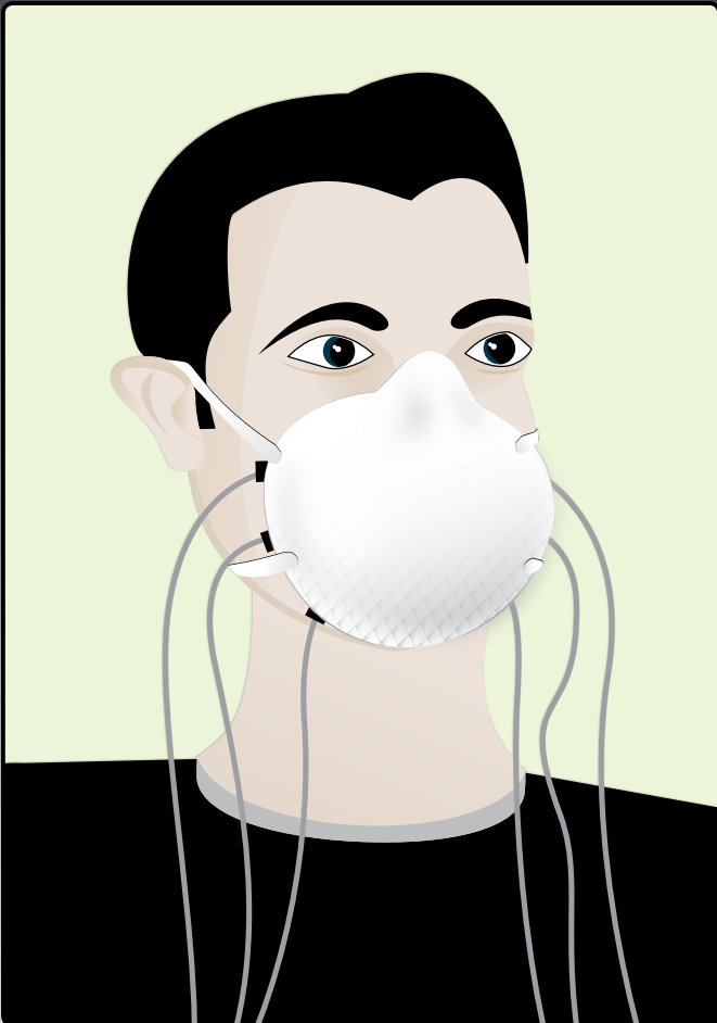
Example of Tactilus Free Form® being used for face mask sealing pressure measurement
