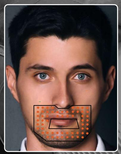
Tactilus® is a flexible textile matrix-based tactile surface sensor—essentially an "electronic skin" that records and interprets pressure distribution and magnitude between the surface of the face mask and skin and assimilates the collected data into a powerful Windows® based tool kit. Each Tactilus® sensor is carefully assembled to exacting tolerances and individually calibrated and serialized.
