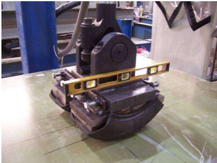
Figure 6.15 Fatigue test on FRP deck using simulated tire patch
