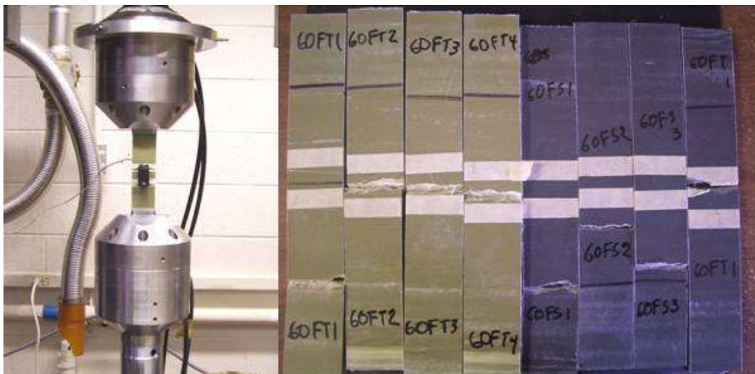
Figure 6.5 Transverse tension fatigue test with plate samples
