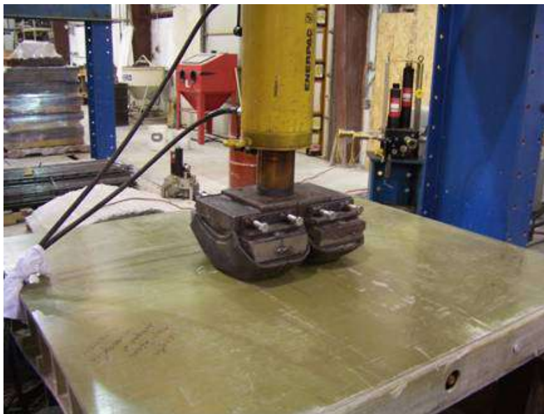
Figure 6.1 Failure Test setup for 5ft by 6 ft specimen
