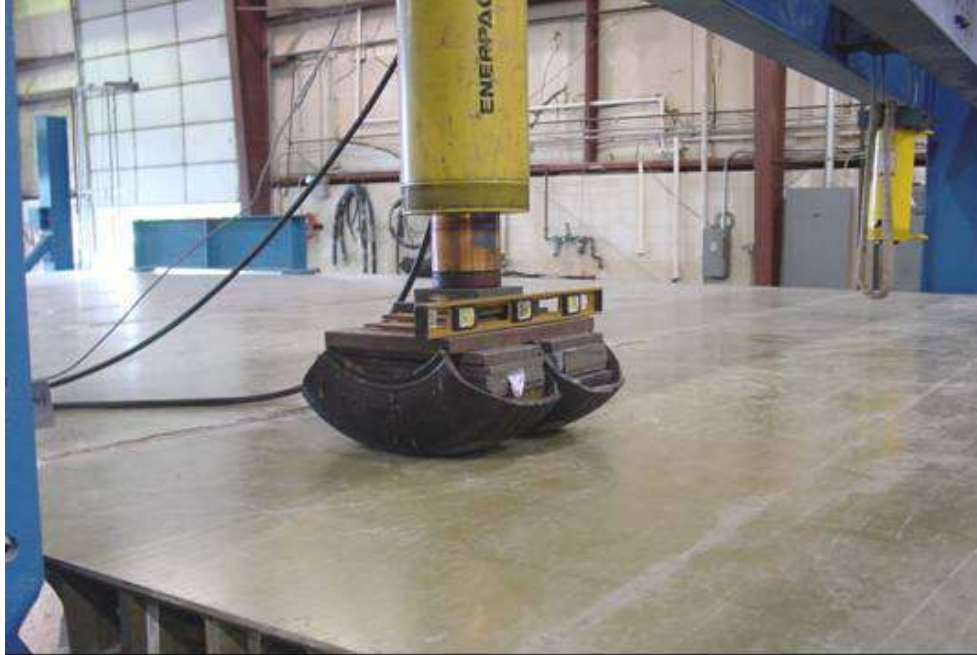
Figure 5.16 Failure test setup
