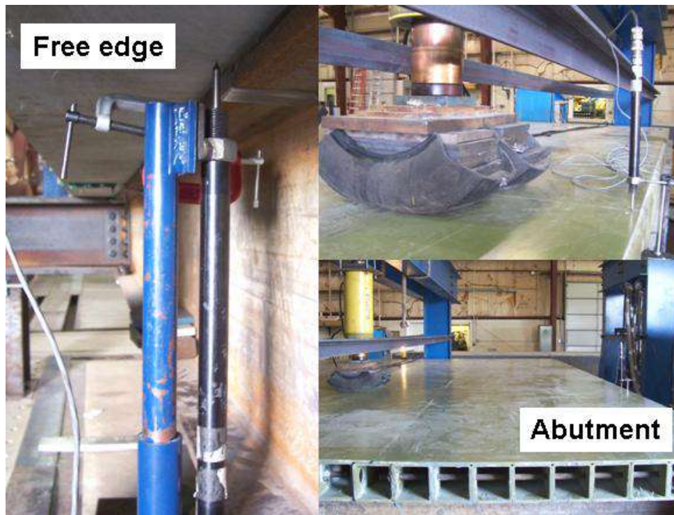
Figure 5.14 Uplift test at free edge for loading near or away from abutment
