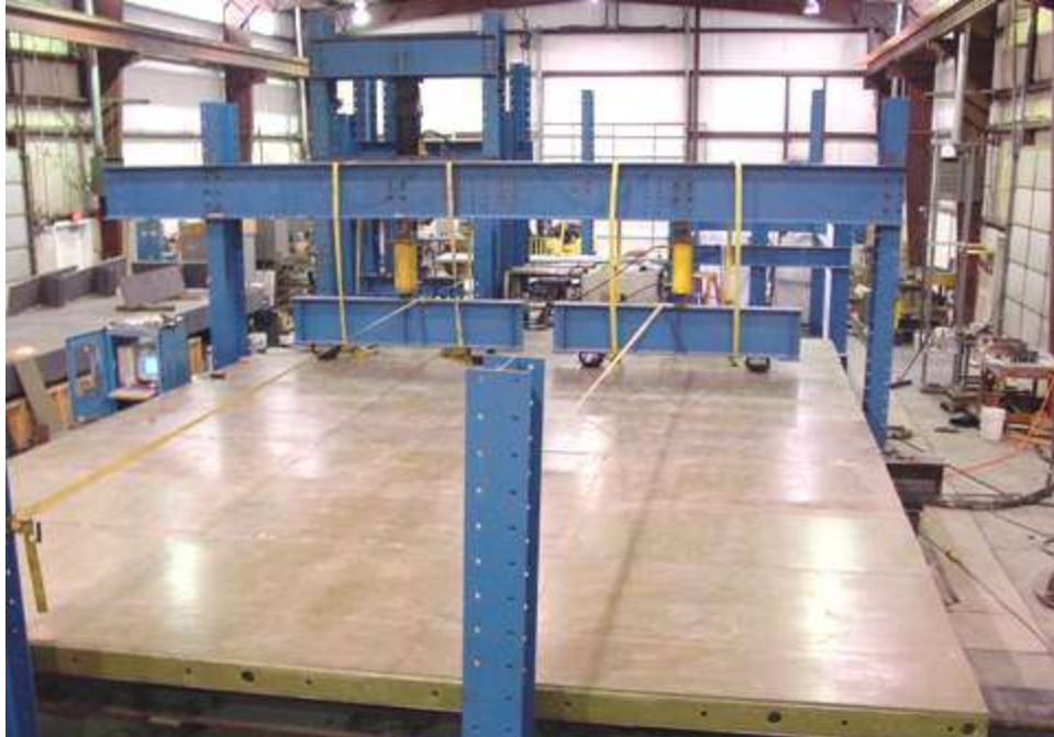
Figure 5.7 Experimental Set-up for service load test
