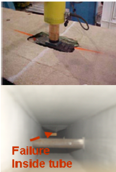
Figure 16 Failure using steel patch [19] and Tire Patch [18]
