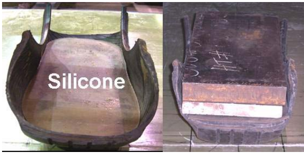
Figure 4 Proposed Simulated Tire Patch with hyper elastic silicone
