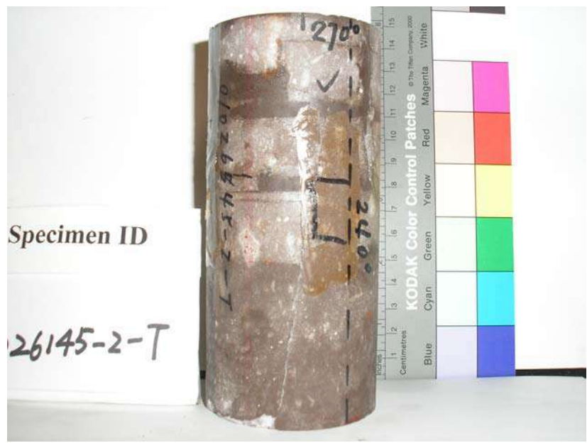
Figure 1.5.3 Specimen after triaxial test, specimen ID 01026145-2-T
