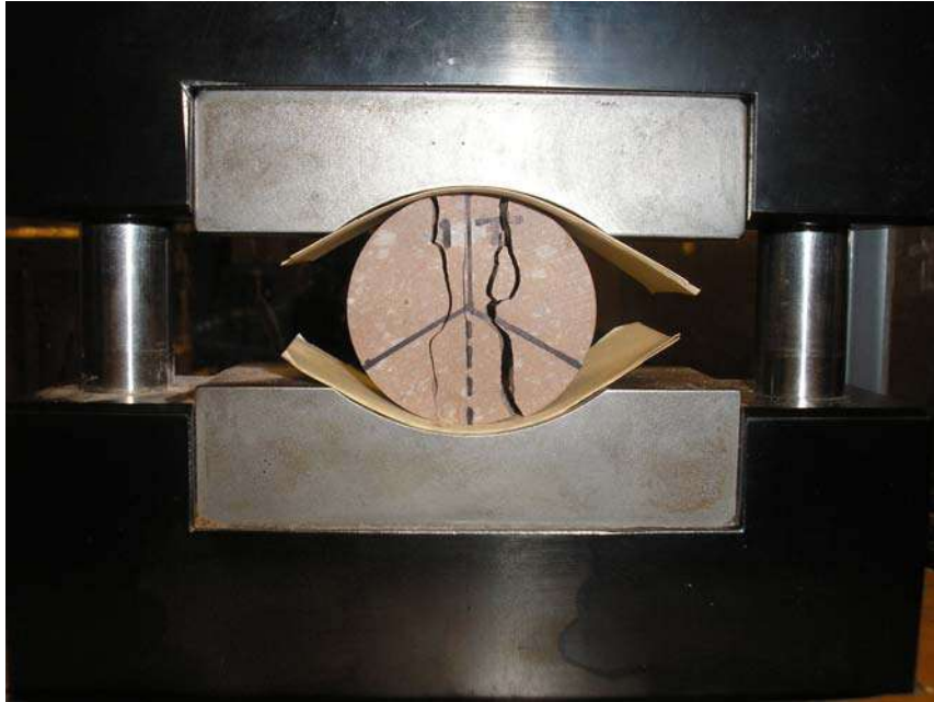
Figure 2.5.9 Specimen after Brazilian (indirect tensile strength) test, specimen ID 01026209-4-B
