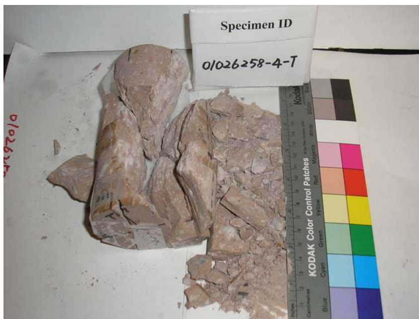
Figure 1.5.8 Specimen after triaxial test, specimen ID 01026258-4-T
