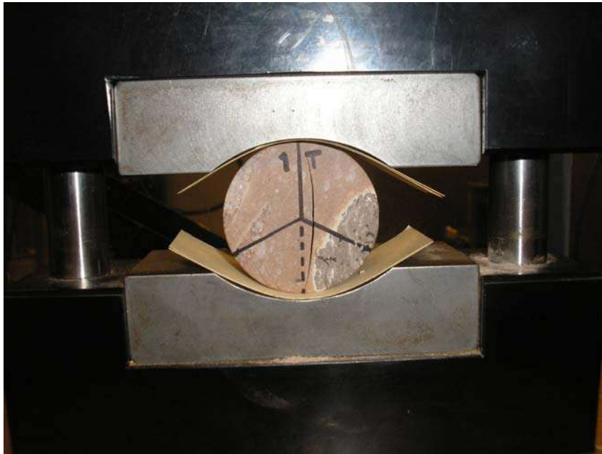
Figure 2.5.10 Specimen after Brazilian (indirect tensile strength) test, specimen ID 01026209-3-B
