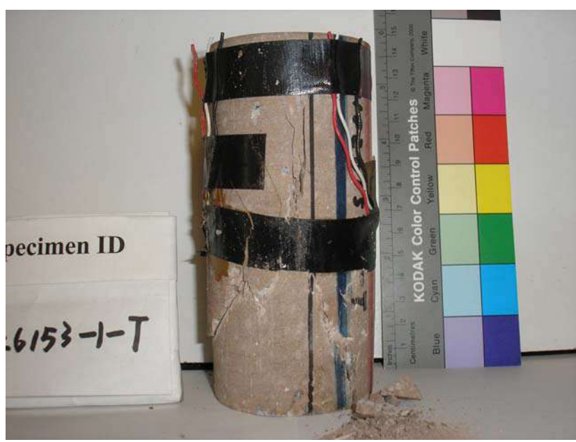
Figure 1.5.4 Specimen after triaxial test, specimen ID 01026153-1-T
