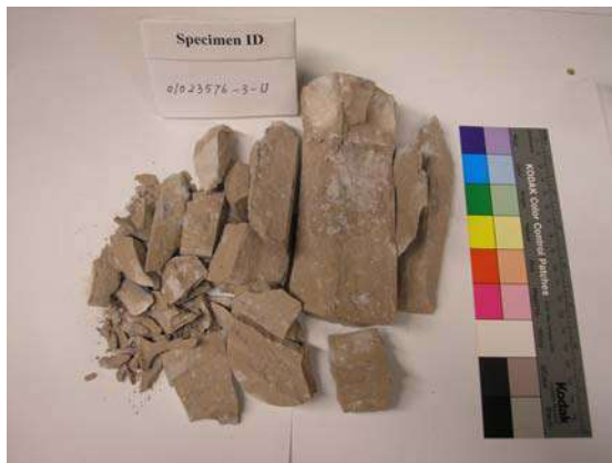
Fig. 5.1: Typical failure at low strain rate (Strain rate= 1.10\text{e-}8 )
