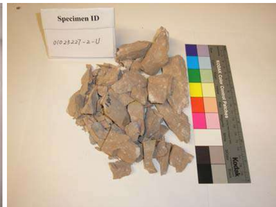
Fig. 5.2: Typical failure at high strain rate (Strain rate= 8.85\text{e-}3 )
