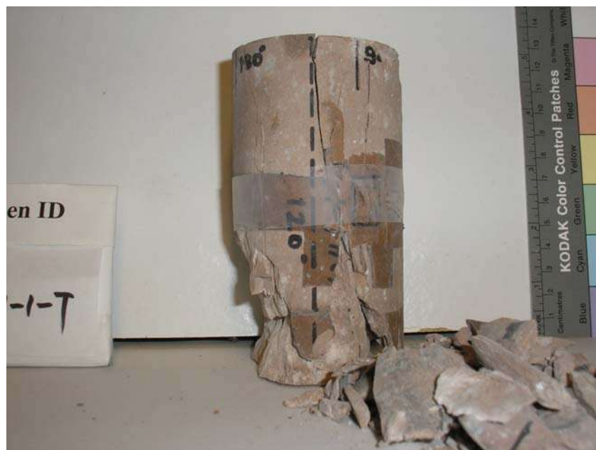
Figure 1.5.7 Specimen after triaxial test, specimen ID 01026241-1-T
