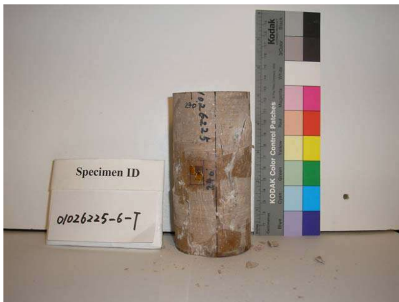
Figure 1.5.5 Specimen after triaxial test, specimen ID 01026225-6-T
