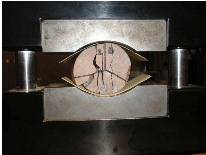
Figure 2.5.8 Specimen after Brazilian (indirect tensile strength) test, specimen ID 01026206-1-B
