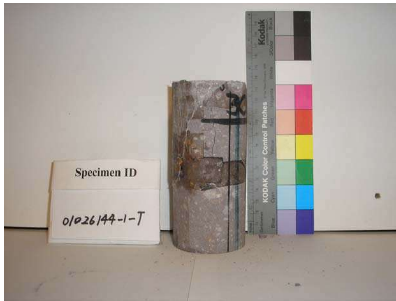
Figure 1.5.1 Specimen after triaxial test, specimen ID 01026144-1-T
