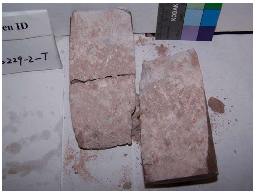
Figure 1.5.6 Specimen after triaxial test, specimen ID 01026229-2-T
