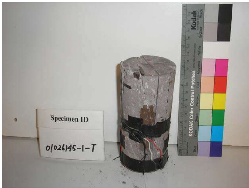
Figure 1.5.2 Specimen after triaxial test, specimen ID 01026145-1-T
