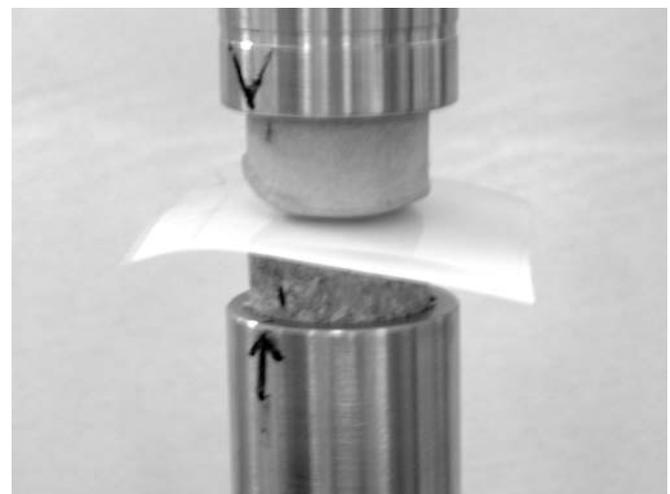
**Fig. 2** The experimental set-up for contact pressure measurement
