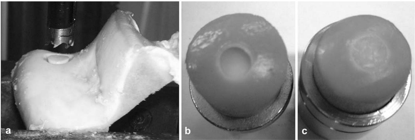
**Fig. 1** Specimen preparation: **a** cylindrical specimens are obtained from the condyles of fresh bovine knees, **b** simulated 12-mm diameter full-thickness cartilage lesion, **c** the lesion filled with fibrin glue
