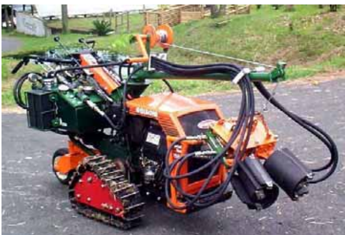
Figure 2 -- Trunk shaker with multidirectional pattern for coffee trunks (VITAC-1) developed at CENICAFE (2001). (Picture source García, 2001)
