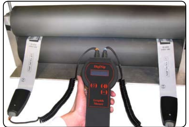
Diginip sensor elements placed between two contacting rollers
