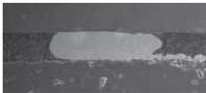
Fig. 5: Cross-section of a gold stud bump, with the top surface flattened by pressure
