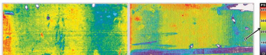
Topaq® pressure analysis of the threaded roll set (l) and the pretension roll set (r)
