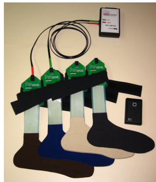
Tactilus® insole sytem hardware
