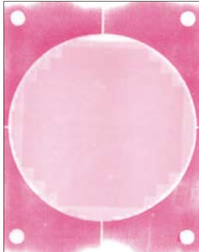
Insufficient pressure was applied to wafer area.
