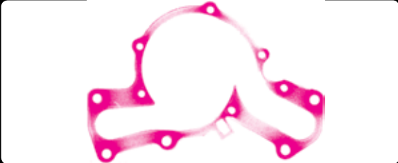
Uneven / Insufficient Loading
