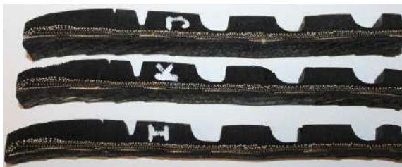
Fig. 8. Specimens of tire 245/40 R18 with transverse direction with different width for tensile and bend tests
