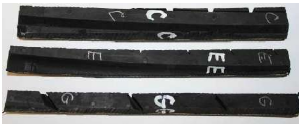
Fig. 7. Specimens of tire 245/40 R18 with longitudinally direction with different width for tensile and bend tests
