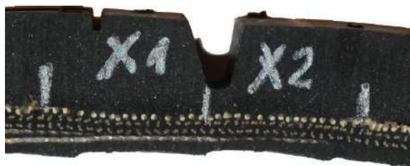
Fig. 2. Structure of cross section of tire-crown of radial tire for passenger car (full colour version available online)
