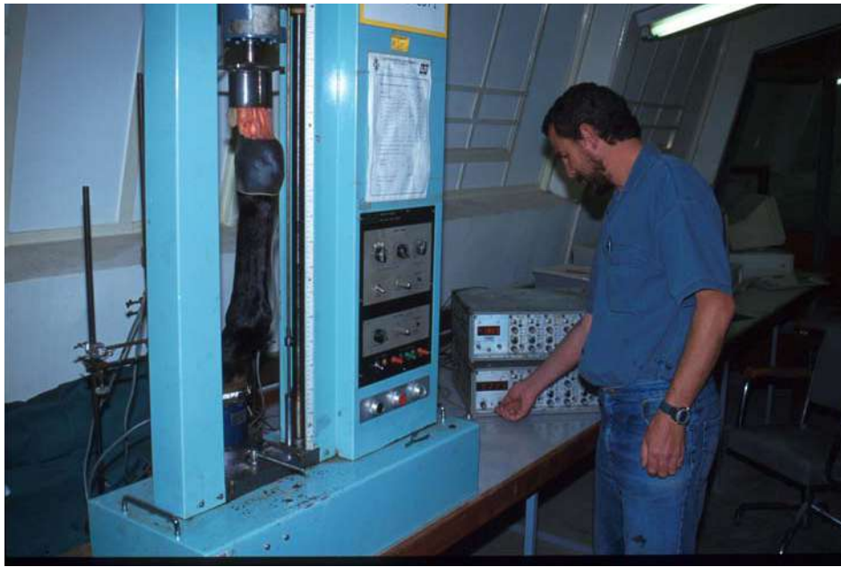
Figure 7: A photograph showing the experimental set-up for the measurement of the load distribution on the solar surfaces and hoof walls of cadaver limbs with partially removed hoof walls and reverse shoes and polystyrene pads applied to them.
