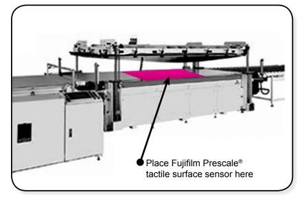
Instantaneously and permanently the film captures both the pressure distribution and magnitude that occurs between the contacting surfaces.
