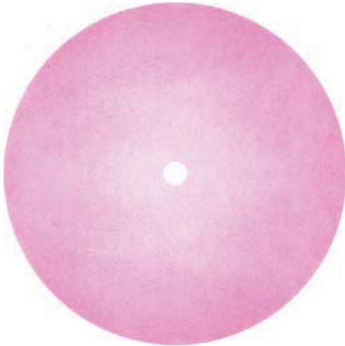
Figure 5: Good pressure distribution
