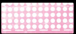
HEAT SEALING Non-uniform Platen Contact / Parallelism Issues
