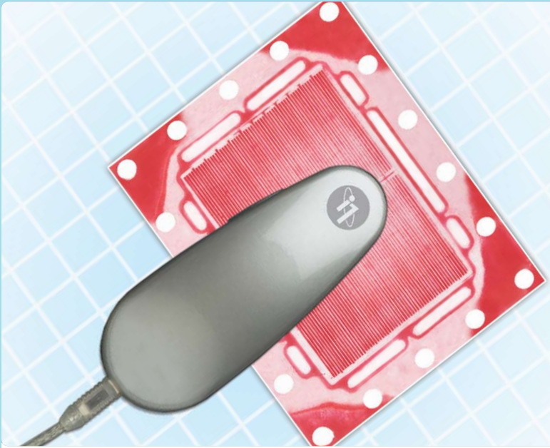
PointScan ® unit pictured atop a pressure indicating film image of a fuel cell
