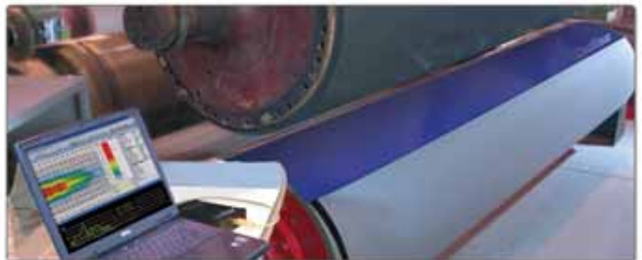
Actual sensor positioned in a nip ● Tactilus® software displayed on laptop
