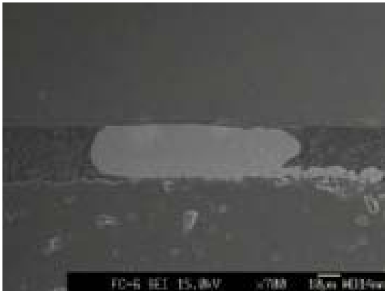
Figure 5. Cross-section of a coined gold stud bump connection.
