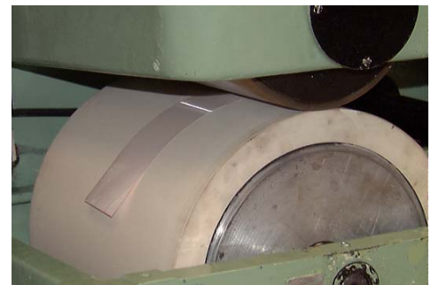
Figure 4 Film strip passing through the threaded roll set.
