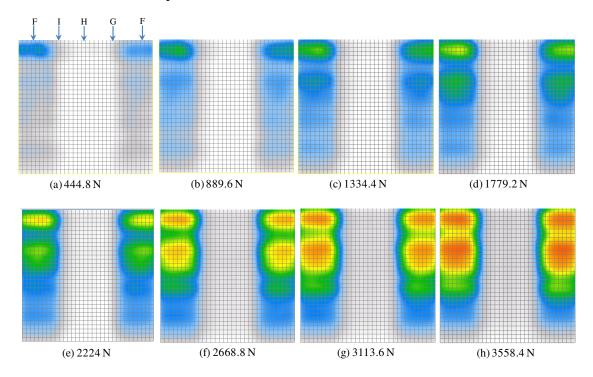
Fig. 7: Soil-pile interaction pressure measured at depth ranging from 43.1 cm to 86.1 cm at several stages during the test.
