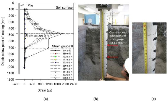
Fig. 6: Strain profile and pile after testing, (a) strain profile along the length of the pile, (b) pile after test with marked cracks, and (c) close view of the cracks with marks showing the locations of strain gauges 6 and 8.
