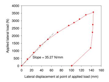
Fig. 5: Measured lateral load vs. lateral displacement of the test pile.
