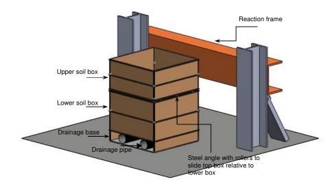
Fig. 2: Setup of Soil-Structure Interaction facility at Lafayette College.
