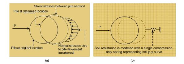
Fig. 1: Soil-pile foundation interaction for active piles, (a) stresses distribution around active pile case, and (b) modeling soil reaction or resistance to pile movement using compression-only springs (p-y curves).
