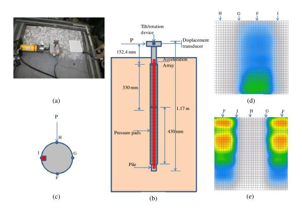
Fig. 4: Test setup and instrumentations of the soil-pile system, (a) soil box with the loading setup, displacement and rotation instrumentation, (b) dimensions and locations of instrumentation, (c) location of reference points used for pressure measurements with the acceleration array embedded on the side of the pile (square shape), (d) top pressure sheet, and (e) bottom pressure sheet.
