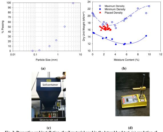
Fig. 3: Properties and installation of soil material used in the lateral load test, (a) gradation of the soil classified at well-graded sand, (b) relative density tests with minimum and maximum density curves conducted at different moisture contents compared with measured dry density and moisture content from the nuclear density gauge, (c) raining the soil from a height of approximately 1.5 m, and (d) nuclear gauge device used to measure soil properties.
