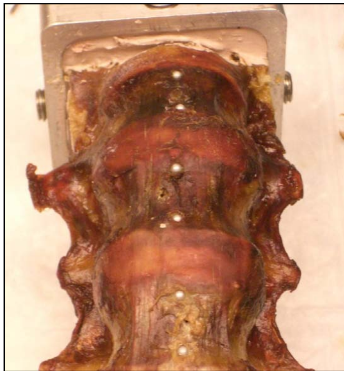
Figure 7: Fiducials Placed on Specimen
