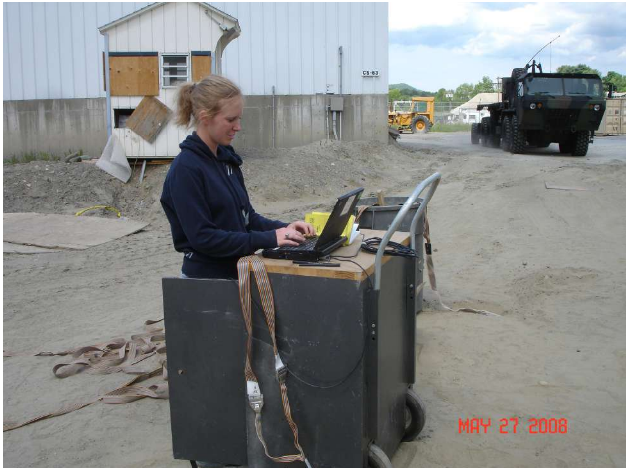
Figure C3. Both buried pads connected to laptop. HEMMT and MDT in upper right, 27 May 2008.
