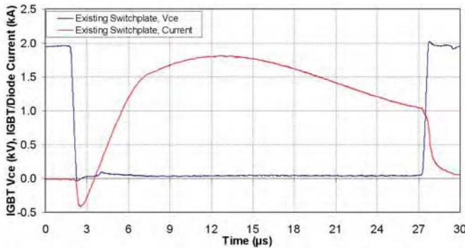
Figure 9. Measured IGBT collector-emitter voltage and IGBT/diode current for both the existing and press-pack switch plates.
