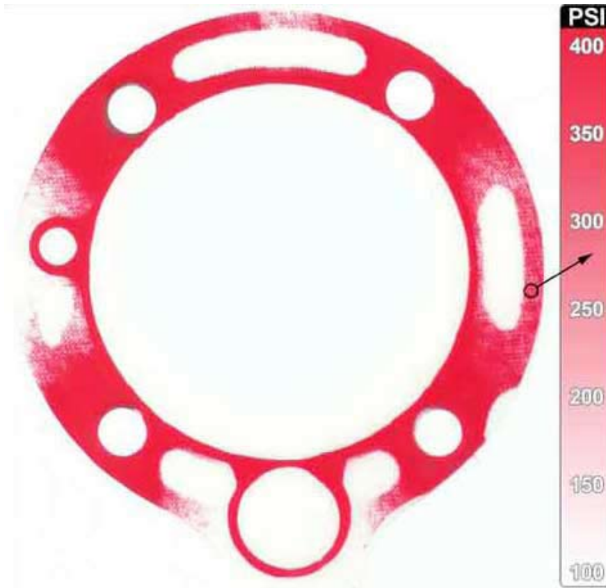
Pressure sensor film reveals gasket's uneven pressure distribution
