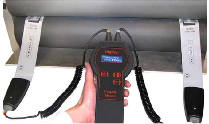
The DigiNip®, from Sensor Products, with its elements placed between two contacting rollers
