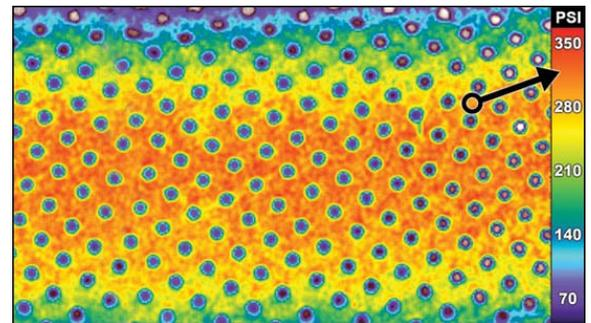
The nip pressure profile as revealed with Sensor Products' Pressurex®
