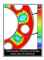
Pressurex reveals pressure distribution and magnitude between mating or impacting surfaces. When placed in the interface, the film changes color in direct proportion to the actual pressure applied. The result is an instantaneous and permanent "topographical" image of pressure magnitude and distribution across the contact area. Precise pressure magnitude is easily determined by comparing color variation results to a color correlation chart (conceptually similar to interpreting Litmus paper).
