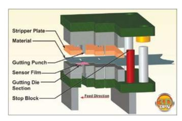
the strip and film. This pressure causes the sensor film's microcapsules to burst, producing an instantaneous and permanent high resolution "topographical" image of pressure variation across the contact area.
