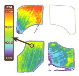
This pressure image of the progressive die reveals that three of the four bumper blocks experienced pressure of 7000 to 20,000 psi, while one block failed to make contact, requiring a shut-height correction
