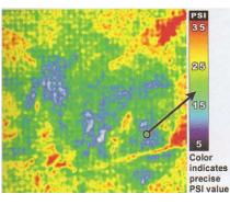
accurately measure map pressure magnitude and distribution. Variations in contact surface pressure are immediately visible by the impression on the film. made spatial resolution film is fine enough expose minute surface defects and other imperfections. The range for Pressurex Zero® is 7.2 -PSI (0.5)kg/cm2).
