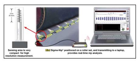
made in real time while the sensors are in the closed, (non-rotating) nip. Problems with alignment, skewing, and crown deficiencies are quickly exposed.
