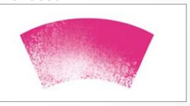
Contact pressure between disc and brake pad is uneven
