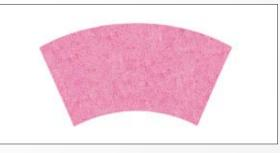
Fit between disc and brake pad is uniform and of optimum pressure
